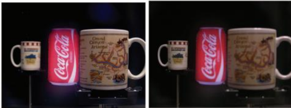
Figure 73. Two real Cups with augmented with a virtual COKE with different focal distance (a)40cm (b)100cm
